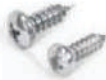
DIN 7981 PHILLIPS PAN HD SELF TAPPING SCREW Dia : M2.2-M6.3 Cold Forge Length : 6.5mm-50mm
