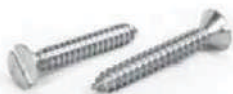
DIN 7972 SLOTTED CSK HD SELF TAPPING SCREW Dia : M2.9-M6.3 Cold Forge Length : 6.5mm-50mm
