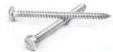
DIN 7971 SLOTTED PAN HD SELF TAPPING SCREW Dia : M2.9-M6.3 Cold Forge Length : 6.5mm-50mm
