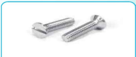
DIN 963 SLOTTED CSK SCREW Dia : M3-M8 Cold Forge Length:10mm-50mm
